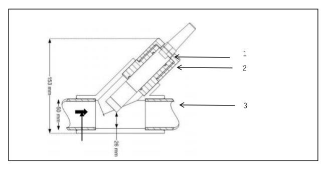
Mounting system for dissolved oxygen sensor (PF-ACC-C-00224)
