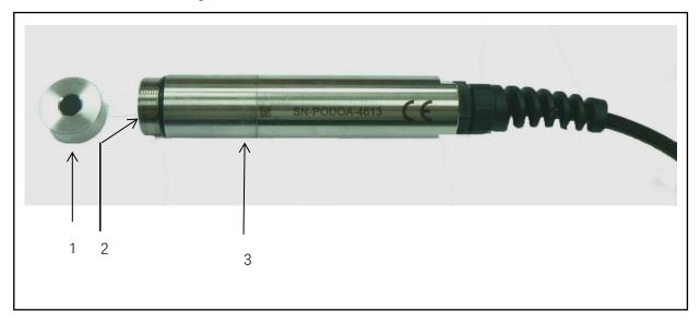
1 Unscrew the stainless steel DODISK (1) from the sensor body with measurement electronics (3). When doing so, ensure that the optical window (2) of the sensor is not touched.
