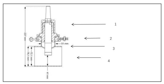
Mounting system for dissolved oxygen sensor (PF-ACC-C-00227)
