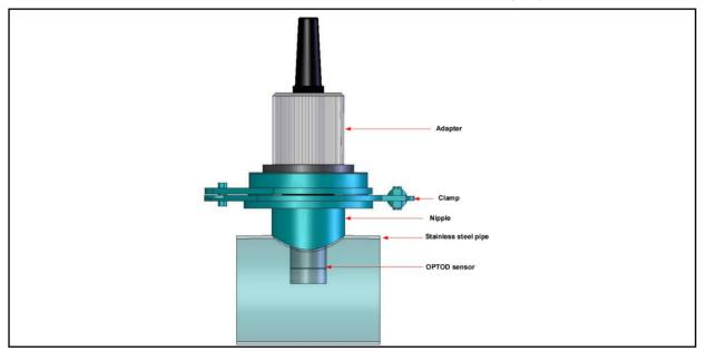
1 After welding the clamp on the stainless steel pipe, remove the clamp from the system and remove the PVC adapter.
