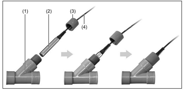
1 Unscrew the union nut (3) from the PVC flow fitting (1).
