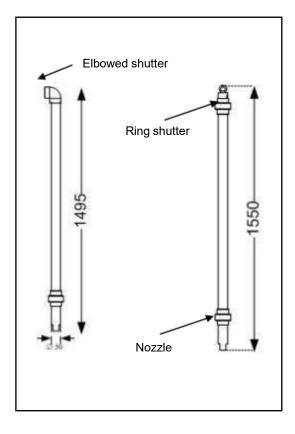
The short pole is available in 2 versions: - version with elbowed shutter. The nozzle of support is included in the offer.
