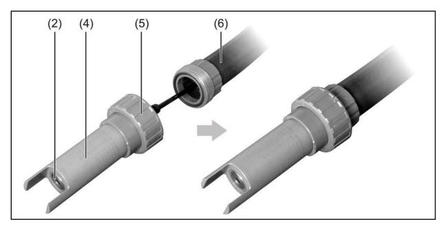
1 Insert the sensor (2) into the nozzle (4) as far as the stop.
